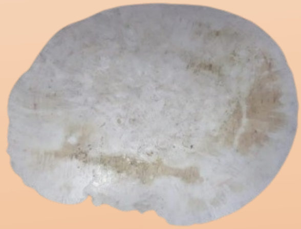
Final Sheets made using Sheet Making Machine from waste Bottle
