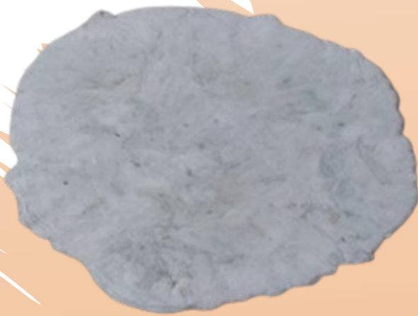
Final Sheets made using Sheet Making Machine from waste Bottle
